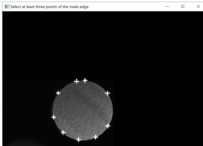
Figure 7: Example of pupil 1 edge fitting procedure by user clicking
