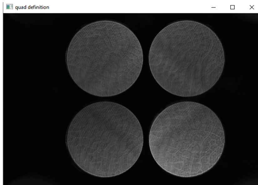
Figure 5: The IDL ® window displays the image and the user is asked to click approximately at the center of the four pupils
