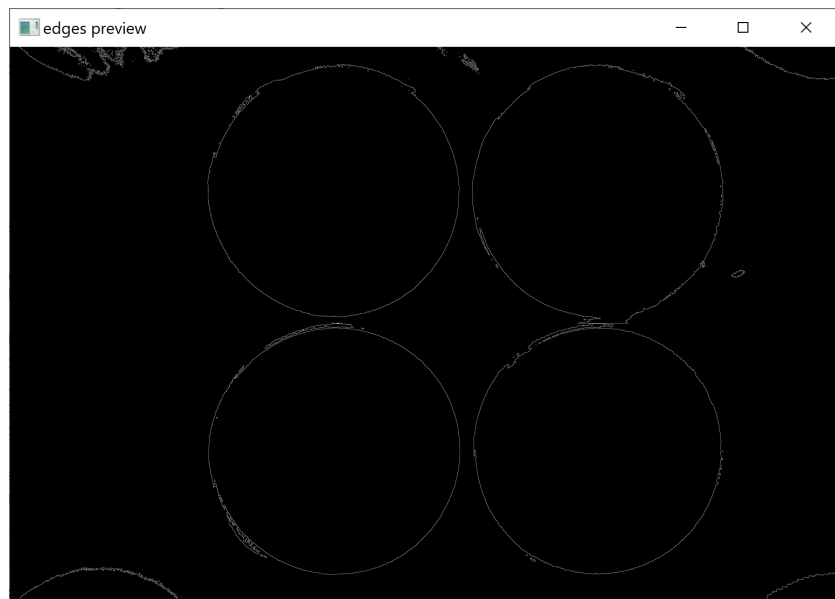
Figure 10: Example of possible edge detection error when using SOBEL
