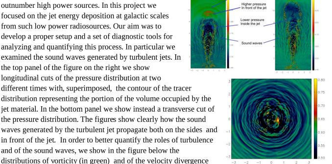
(in pink and orange). The vorticity shows the turbulent jet, while the velocity divergence shows the acoustic field around the jet. There are different mechanisms for the generations of sound waves: the Lightill mechanism (Lightill 1952), fragments of the jet moving at supersonic velocities (Tam & Burton 1984) and the conversion of vortices in waves in the presence of shear flows (Chagelishvili et al. 1997). All these mechanisms are at work in the present situation,
