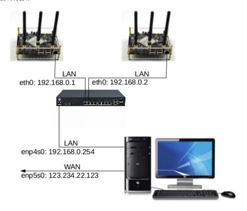
Figure 1: Cluster components, layout and networking
