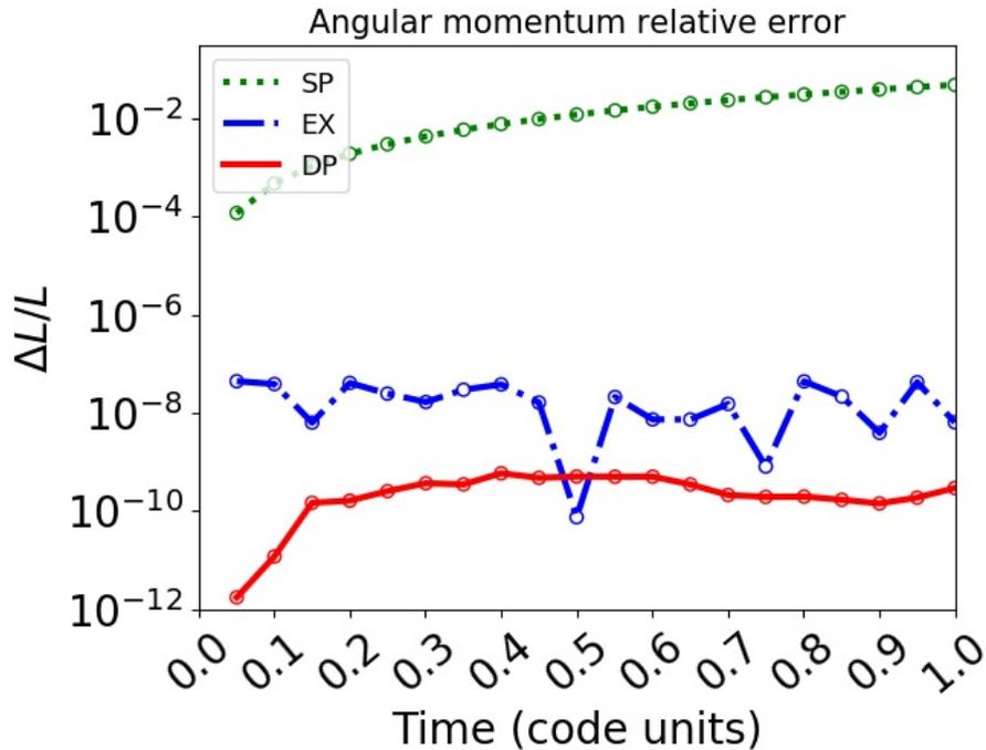
Figure 2: Relative error  $\Delta L/L$  for DP-arithmetic (continuous red line), EX-arithmetic (dot-dashed blue line) and SP-arithmetic (dotted cyan line) as a function of the integration time (in code unit).
