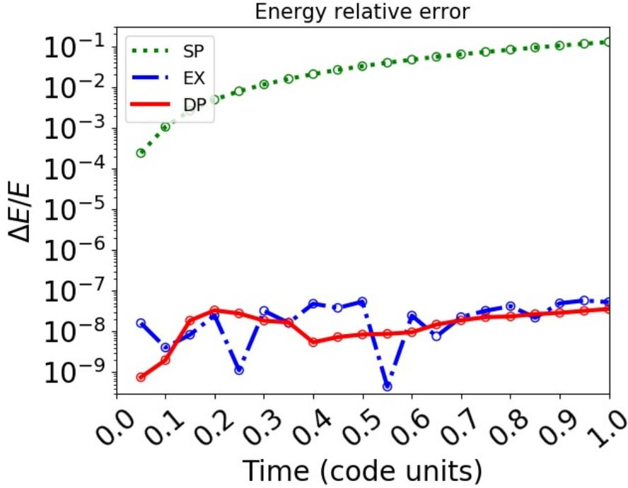
Figure 1: Relative error  $\Delta E/E$  for DP-arithmetic (continuous red line), EX-arithmetic (dot-dashed blue line) and SP-arithmetic (dotted cyan line) as a function of the integration time (in code unit).
